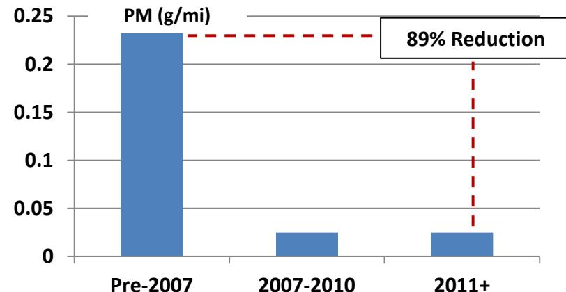
EPA estimates for in-use distance based output. Phase-in for 2004 and 2007 rulemaking is averaged across 2007-2009 and 2010 and beyond respectively. Pre-2007 estimates are based on an estimate of all vehicles in operation before 2007.
