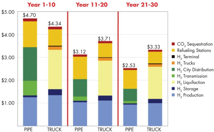
*Our dynamic modeling for California came up with these levelized costs for hydrogen delivered via pipeline and truck over a 30-year planning period.*
