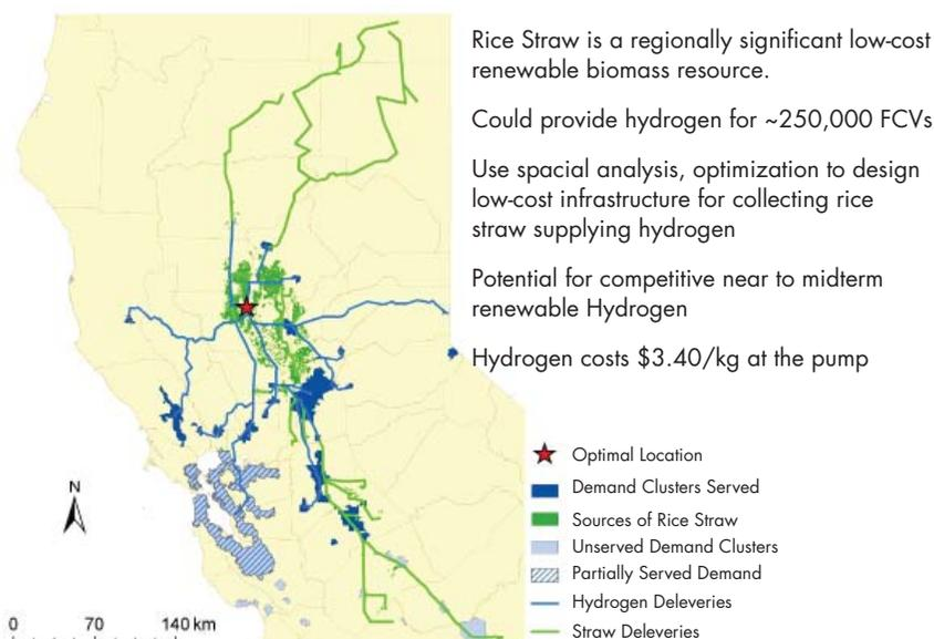
*Parker et al. examined the possibility of using rice straw to make biomass hydrogen in California and found that under certain circumstances it would be possible to reduce the costs of biomass hydrogen through optimal location of production plants and design of delivery systems. Source: N. Parker, Y. Fan, and J. Ogden, "From Waste to Hydrogen: An Optimal Design of Energy Production and Distribution Network," Transportation Research E: Logistics 46 (2010): 534–45.*
