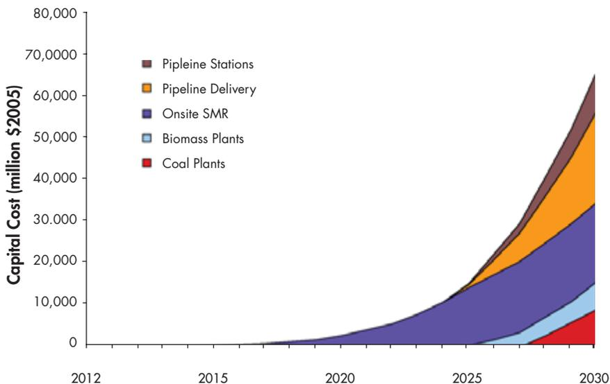
We assume that the choice of supply pathway for hydrogen fuel will vary over time as demand grows and production scales up. On-site SMRs dominate until about 2025, and after that central biomass and coal plants (with CCS) come in along with pipeline distribution systems. Source: J. Ogden and C. Yang, "Build-up of a Hydrogen Infrastructure in the U.S.," Chapter 15 in M. Ball and M. Wietschel, *The Hydrogen Economy: Opportunities and Challenges* (Cambridge, UK: Cambridge University Press, 2009).
