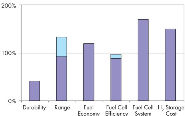
*When we compare the status of current (2010) H<sub>2</sub> technologies in demonstration vehicles and goals set by the U.S. Department of Energy (DOE) for 2015, we can see that current technologies have farthest to go to reach durability, system-cost, and storage-cost goals. The figure at the bottom shows how close the current technology is to the 2015 goal.*
