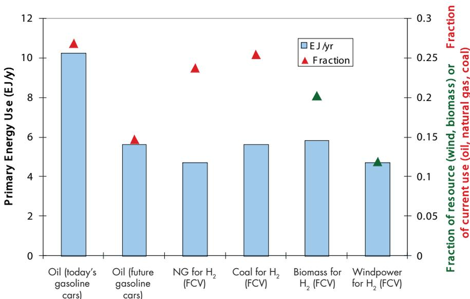
We did a sample calculation of the amount of primary energy needed to make hydrogen for 100 million FCVs in the United States (about 50 percent of the current U.S. fleet or 33 percent of the projected U.S. fleet in 2050). The amount of primary energy required is measured in exajoules ( $10^{18}$  joules) per year by the y-axis on the left. The fraction of the available annual resource (for biomass and wind) or the current use (for coal or natural gas) is measured by the y-axis on the right.
