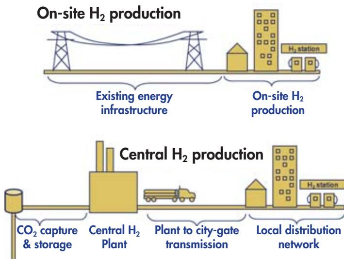
Options for producing and delivering hydrogen include on-site production and central production. Source: C. Yang and J. Ogden, "Determining the lowest-cost hydrogen delivery mode," *International Journal of Hydrogen Energy* 32 (2007): 268–86.
