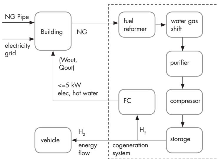
*A typical tri-generation system simultaneously provides home electricity and heat along with hydrogen for a vehicle.*
