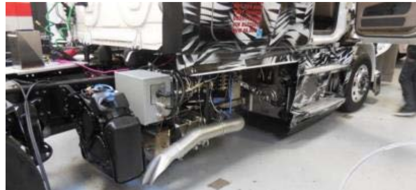
Waste-Heat Recovery system on A-sample SuperTruck prototype.
