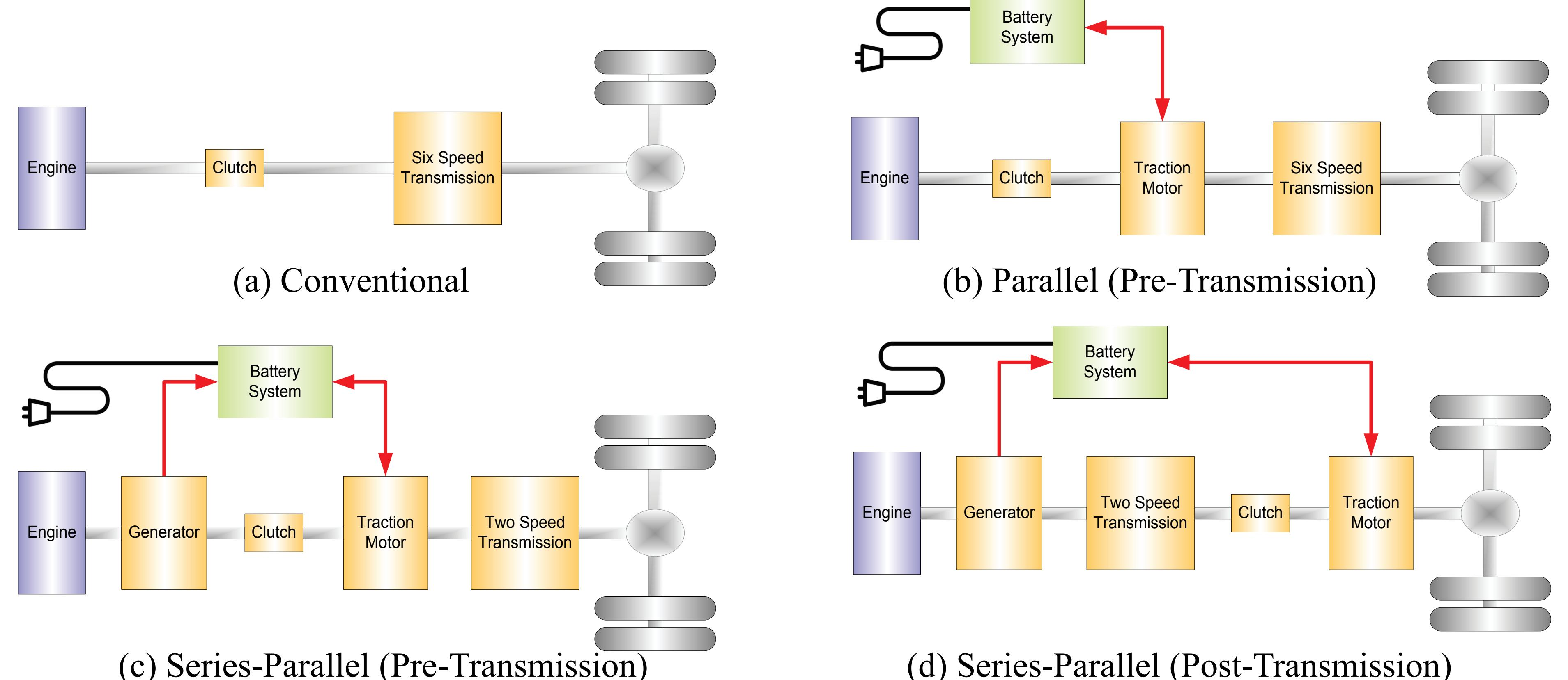
Figure 1: Delivery truck powertrain architectures
