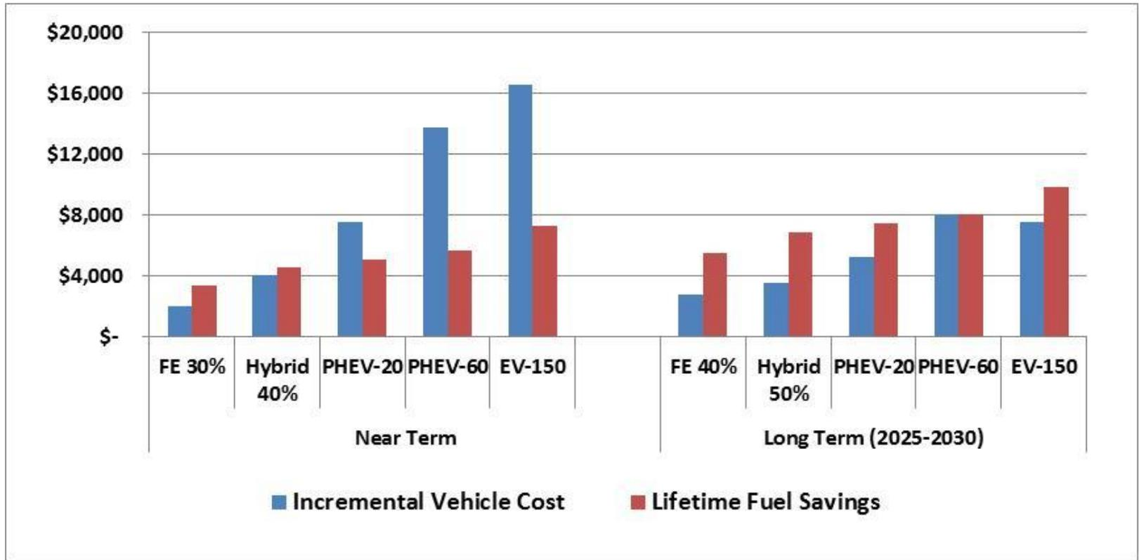
**Notes:** "FE 30%"=fuel economy improved by 30% in L/100km; "PHEV-20"= plug-in hybrid with 20 km electric range; fuel savings estimated over 160k kms of driving; all related to a base gasoline vehicle of 9 L/100km; oil prices \$100/bbl near term, \$130/bbl long term; battery costs decline over time from \$600 to about \$300/kWh
