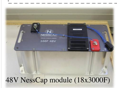
The optimum duty cycle for the batteries is that they provide the average power and the supercaps meet most of the peak discharge pulses during accelerations and accept the charging pulses during regenerative braking. (in other words, the supercaps load-level the battery).
