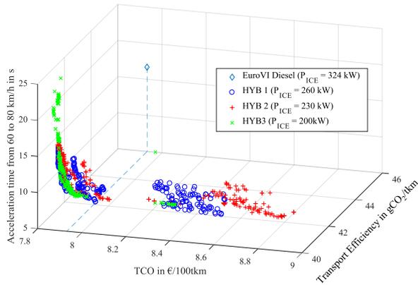
Figure 4. Pareto optimal solutions of the hybrid configurations with discrete engine power levels in the 150<sup>th</sup> generation of optimization
