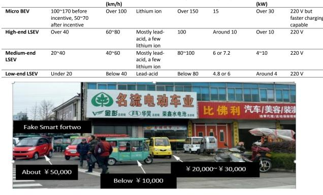
Figure 6: Three Categories of LSEVs vs Micro BEVs
